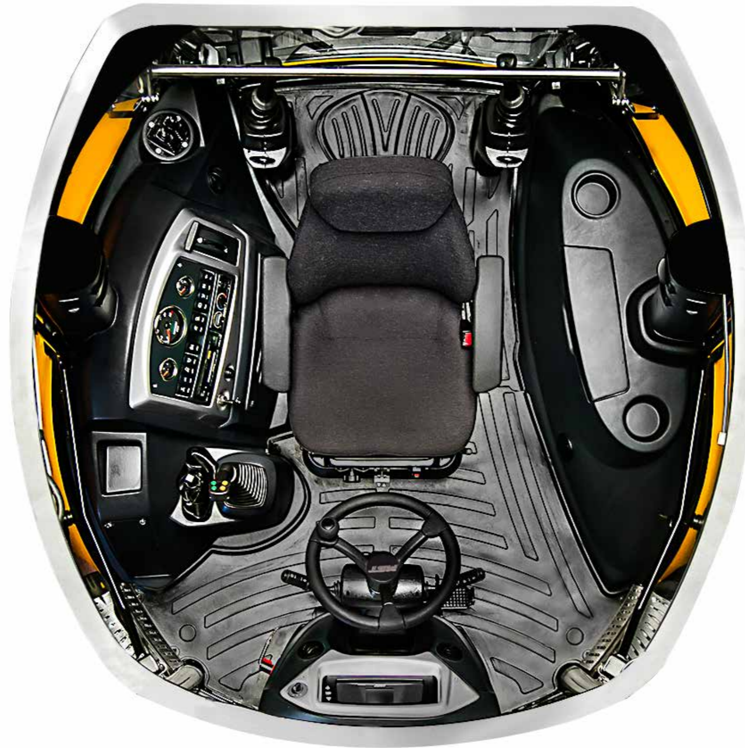
Operator seat with anti-fatigue with air suspension for heavy-duty use over extended periods.
