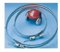
The unit lengths are connected together by pulling the end of one duct over the end with steel ring of next duct. Around the joint, a SWEDFAN coupling clamp is positioned. The coupling clamp is made of 1.5 mm profiled galvanized steel with mounted threaded crank. The joint is sealed by tightening the coupling clamp using the threaded crank.
