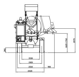
LOADING SHOVEL: Effective capacity 600 liters, self articulated complete with hydraulic opening gate. 6 bukets only per batch
